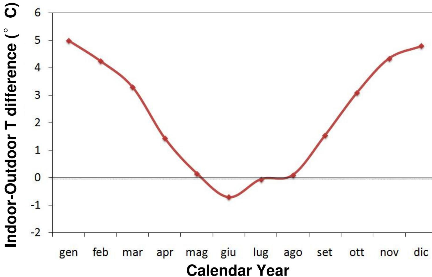
An example of measured indoor – outdoor temperature difference in Northern Italy
