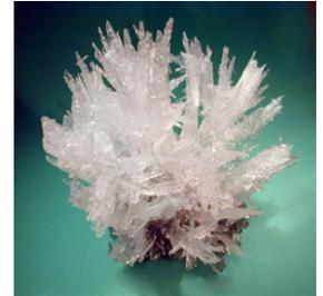
Mirabilite exerts a very high crystallization pressure on the pore wall causing damage of the stone. Moreover, the transient stress can remain for a long period of time since the relaxation process is slow (Espinosa et al., 2008).
