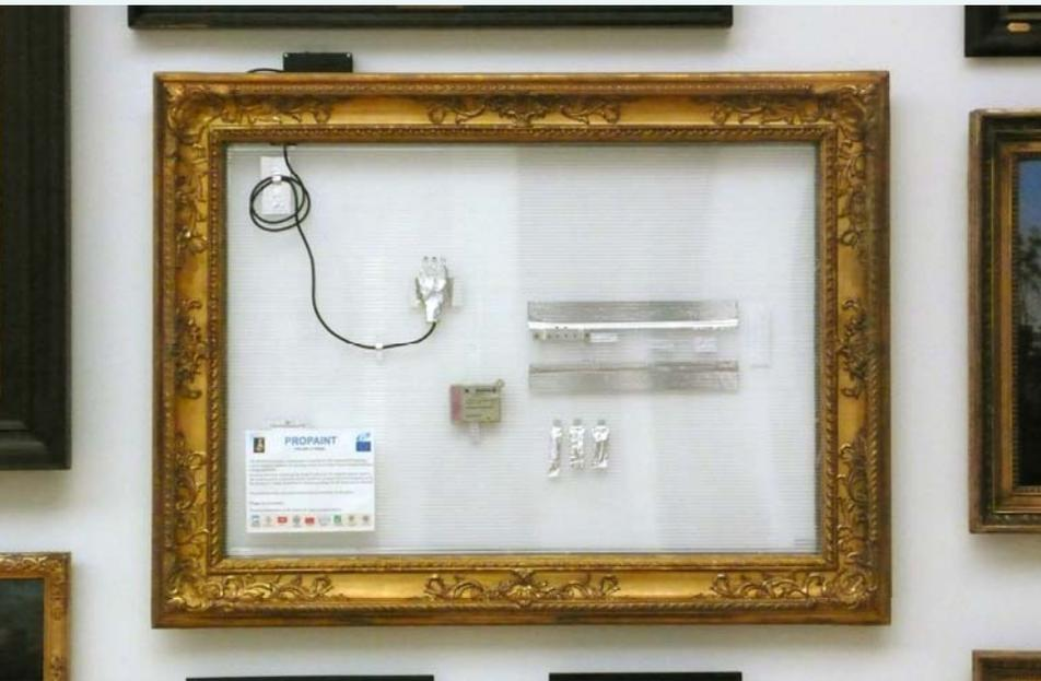
***Lead coated PQC Dosimeters for continuous monitoring for volatile organic acids.***
