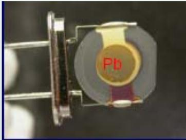
Change (%) is calculated from the frequency shift  $\Delta f(\text{Hz})$  relative to the original frequency of the crystal ( $F_0(\text{kHz})$ ) after coating
