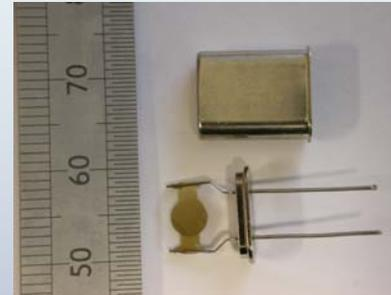
**The PQC-dosimeter responds to the cumulative dose received and can be responsive to (1) volatile organic acids or (2) photooxidising effects.**
