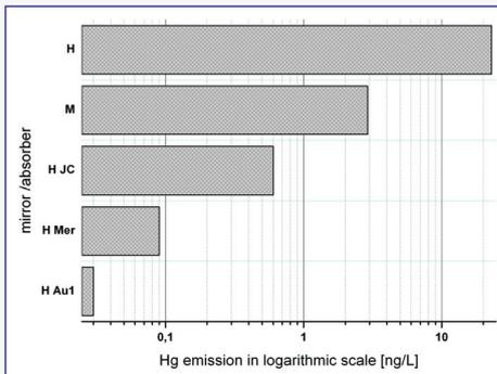
Logarithmic presentation of the analytical results for the emission of mercury from historical (H) and "modern" (M) tin amalgam mirrors and the effects of iodized activated carbon (JC), Mercurisorb<sup>®</sup> (Mer) and gold sputter-coated paper (Au) as adsorbing agents.
