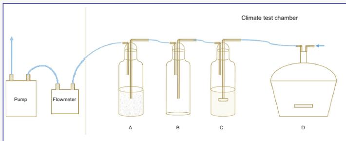
Schematic of the mercury enrichment set-up
