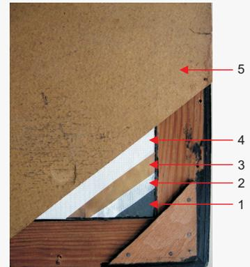
1: tin amalgam mirror in a historic frame, 2: acid-free Tyvek<sup>®</sup> fabric, 3: gold sputtered paper, 4: acid-free Tyvek<sup>®</sup> fabric, 5: back board
