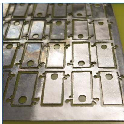
Fig. 2: Grid cut and partly cleaned lead indicators.
