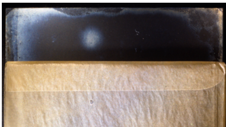
Figure 16. Silver gelatin glass negative. Cueni study collection (□1910). Spot of silver mirroring connected with a black spot on the storage glassine envelope. For purpose of showing this effect, the plate is shifted to the top.
