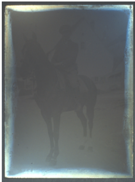
Figure 4. Silver gelatin glass negative. Cueni study collection (□1910). The mirroring extension is smaller at the plate corners than at the centre of the sides.
